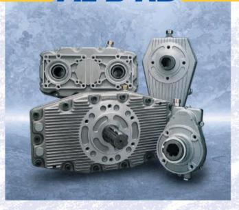
Gear boxes are mainly used to connect hydraulic pumps to agricultural tractors power takeoffs. The P.T.O. speed (standardized at 540 r.p.m.) is thus increased in order to maximize the pump efficiency.
